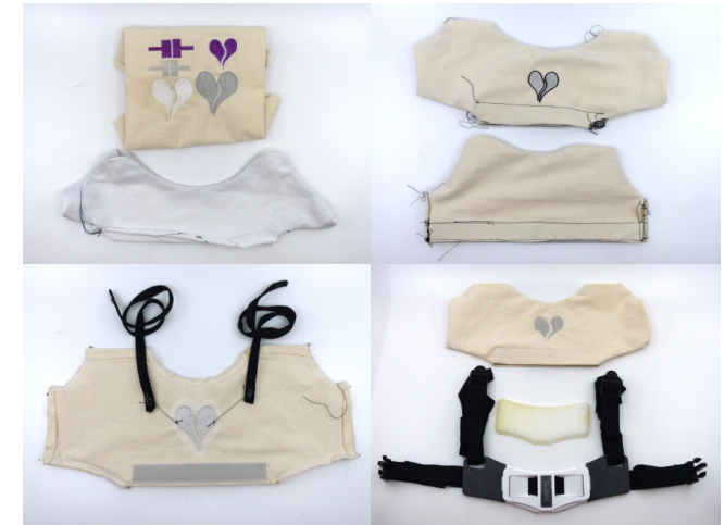
Fig. 11: Test embroidery (tl). First fabric enclosure and embroidery prototype (tr). Hidden steel thread attached to conductive embroidery (bl). Final chest-plate components (br).
